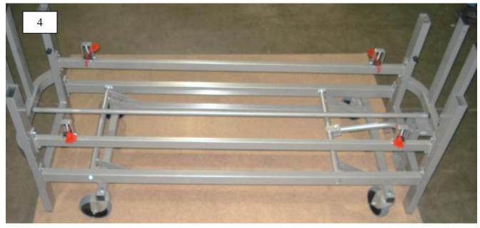
**Step 5:** Prepare tops for assembly to wheelbase
