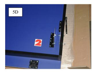
5E: Ensure that all the bolts and nuts are tightened properly. Repeat this assembly for the other table top.
