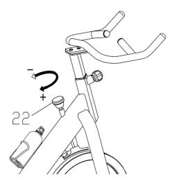
Use the Tension/Brake Knob on Main Frame to adjust the resistance for exercises.
