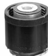
**12030 threaded system testing adapter** is required to test most BMW and Land Rover cooling systems with a threaded filler neck. (Vehicles using Stant® 10246, 10247 radiator caps).
