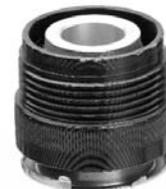
**12028 system testing adapter** is required to test 1990 and newer Volkswagen cooling systems with a threaded filler neck. (Vehicles using Stant® 10243 radiator cap). Thread specifications M 57 x 3.
