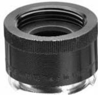
**12018 threaded adapter** is required to fit some Volvo, Saab and late model Renault cooling systems with a threaded filler neck on the expansion tank. Thread specifications M 43.2 x 3. (Vehicles using the Stant® 10244, 10245, 10252, and 10260 radiator cap).
