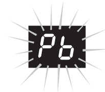
Figure 9: Display will flash if pan is not correctly centered or if no pan is on the cooking zone
