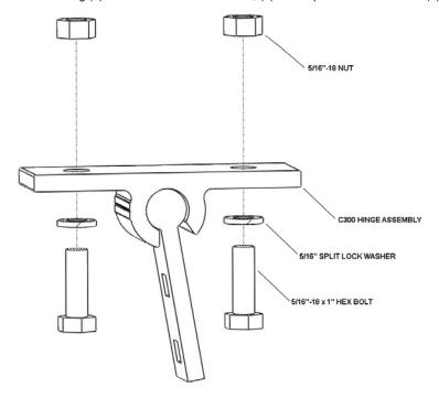
Assemble the C300 hinge leg as shown using (2) 5/16"-18 x 1" hex head bolts, (2) 5/16" split lock washers and (2) 5/16"-18 nuts.
