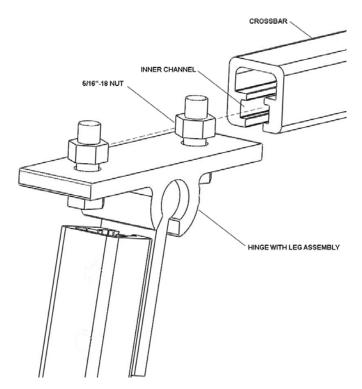
Slide in (1) 5/16"-18 nut into the inner channel of the crossbar on each end as shown below.
