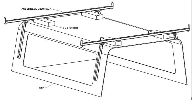
Check to make sure the front and rear crossbar assemblies are level with each other. Adjust if needed.
