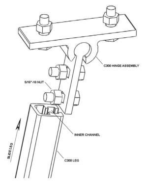
Slide the C300 leg so that the end of the leg is 1/8" from the hinge base. Tighten the 5/16"-18 x 1" hex bolts.
