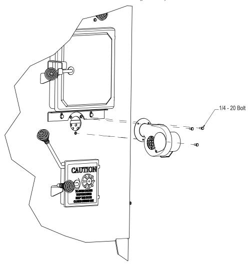
6. Attach the draft blower shield to the bracket that is mounted on the front of the furnace, above the draft blower, using the  $\frac{1}{4}$ -20 x  $\frac{3}{4}$  inch bolts and nuts provided.
