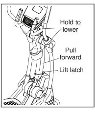
Next, hold the handle on the front stabilizer and lift the elliptical until it will roll on the wheels (not shown) on the rear stabilizer. Then, carefully move the elliptical to the desired location, and lower it to the floor.
