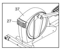
Screws (not shown) from the Top Shield (37), and then use a flat screwdriver to pry the Top Shield upward off the elliptical.
