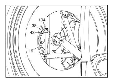
Then, plug in the power cord and turn the left crank arm for a moment. Repeat the procedure above, if necessary, until the console displays correct feedback. Then, reattach the left disc.
