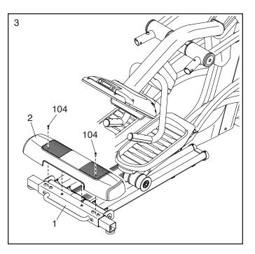
4. With the help of a second person, place some of the packing materials (not shown) under the front of the Frame (1). Have the second person hold the Frame to prevent it from tipping while you complete this step.
