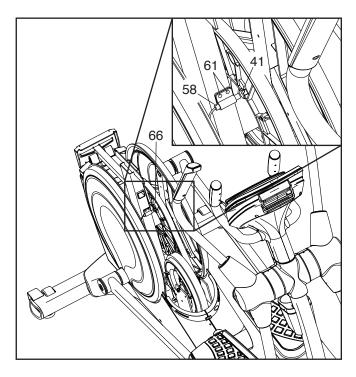
Next, loosen, but do not remove, the two indicated M4 x 16mm Screws (61). Slide the Reed Switch (58) slightly toward or away from the Magnet (41). Then, retighten the M4 x 16mm Screws.
