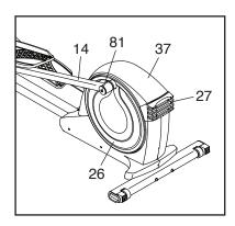
Remove the four M4 x 16mm Screws (not shown) from the Large Storage Foot (27), and then remove the Large Storage Foot. Remove the two M4 x 16mm Screws (not shown) from the Top Shield (37), and then use a flat screwdriver to pry the Top Shield upward off the elliptical. Then, pry the left Pedal Disc (26) off the elliptical.
