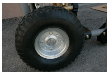
Figure a., axle/washer/wheel/tire assembly
