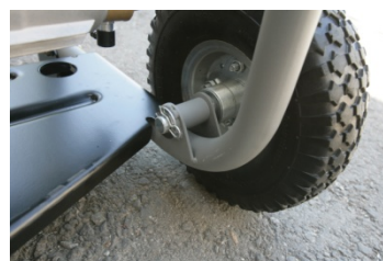
Figure b, insert washer and secure with cotter pin, bend pins so they do not extend past the washer
