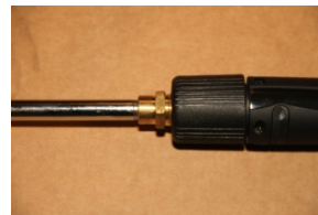
Figure b, tight the nut until the wand is secured fully as shown.
