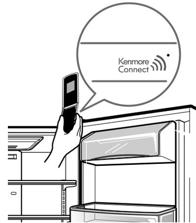
4. Press and hold the Freezer Temp button for three seconds while continuing to hold your phone to the speaker.
