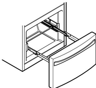
With both hands, hold the center bar and push it in to allow both rails to slide in simultaneously.
