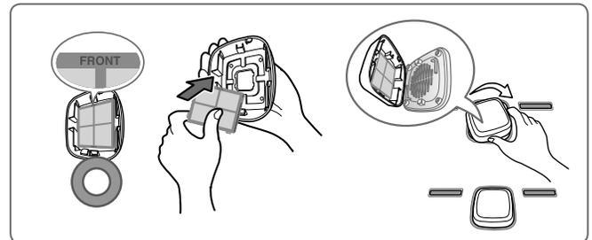
After changing the filter, press and hold the Air Filter button for three seconds to reset the filter sensor.
