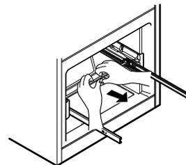
Grasp the drawer on each side and hook the door supports ① into the rail tabs ② located on both sides.
