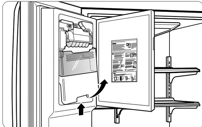
3. To reinstall the in-door ice bin, slightly slant the bin during replacement to avoid contact with the icemaker.
