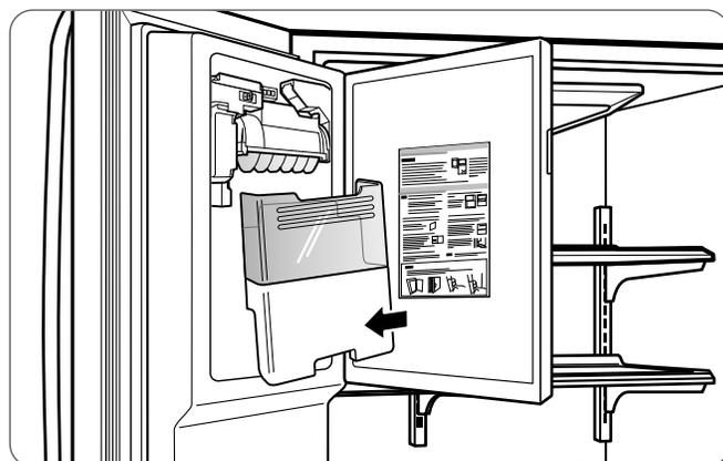
4. Avoid touching the ice-detecting sensor when replacing the bin. See the label on the ice compartment door for details.
