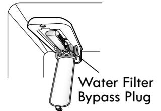
**CAUTION:** DO NOT operate the refrigerator without the water filter or water filter plug installed.
