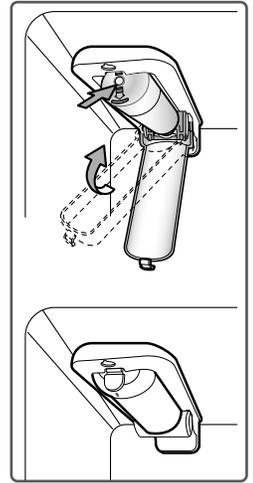
3. After the water filter is replaced, dispense 2.5 gallons of water (flush for approximately 5 minutes) to remove trapped air and contaminants from the system. Do not dispense the entire 2.5 gallon amount continuously. Depress and release the dispenser pad for cycles of 30 seconds ON and 60 seconds OFF.
