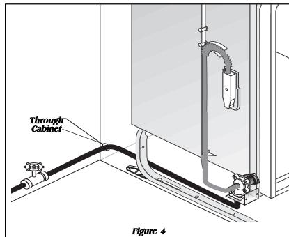
4. Cut water access hole in shaded area in Figure 2. 5. Route water supply line into installation area IMPORTANT: Incoming hot water temperature should be at least 120°F (49°C). Water pressure should be between 20-120 psi.
