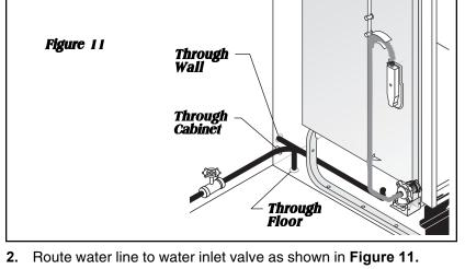
3. While firmly pulling water supply line into 90° elbow, tightly connect water supply to water inlet valve. Supply line must be free of kinks, scales, chips, and lubricants. 4. Turn on water supply and check for leaks.
