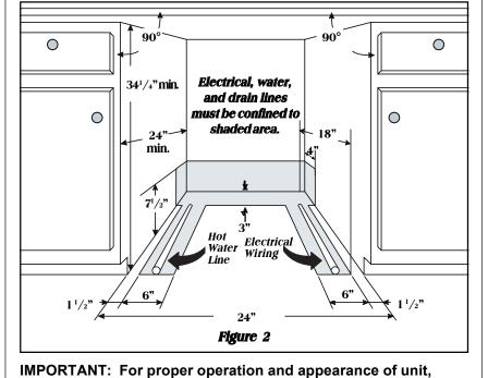
cabinet opening should have dimensions as shown in Figure 2. If unit is to be placed in a corner, there must be at least a 2-inch side clearance to open door.
