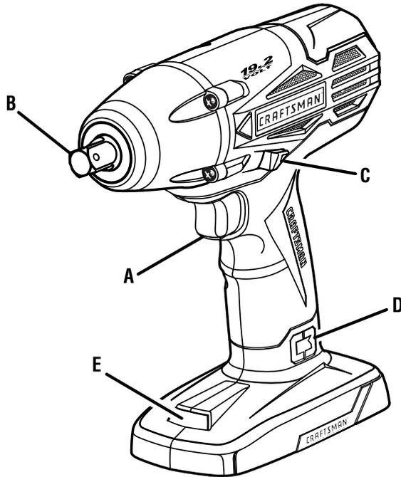
A - Switch trigger (gatillo del interruptor)
