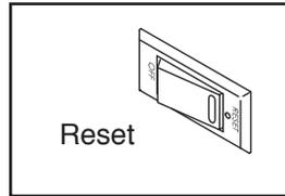
**IMPORTANT:** The console features a display demo mode, designed to be used if the treadmill is displayed in a store. If the displays light as soon as you plug in the power cord and press the power switch into the reset position, the demo mode is turned on. To turn off the demo mode, hold down the Stop button for a few seconds. If the displays remain lit, see THE INFORMATION MODE on page 21 to turn off the demo mode.
