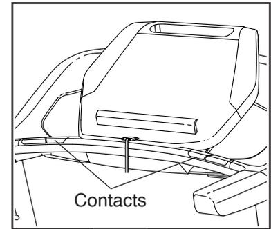
To measure your heart rate, **stand on the foot rails** and place your hands on the metal contacts—**avoid moving your hands**. When your pulse is detected, your heart rate will be shown. **For the most accurate heart rate reading, continue to hold the contacts for about 15 seconds.**
