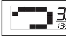
The lower left display can show the elapsed time and the distance that you have walked or run during your workout. Each time you change the incline, the display will show the incline setting for a few seconds. Note: When a workout is selected, the display will show the time remaining in the workout instead of the elapsed time.
