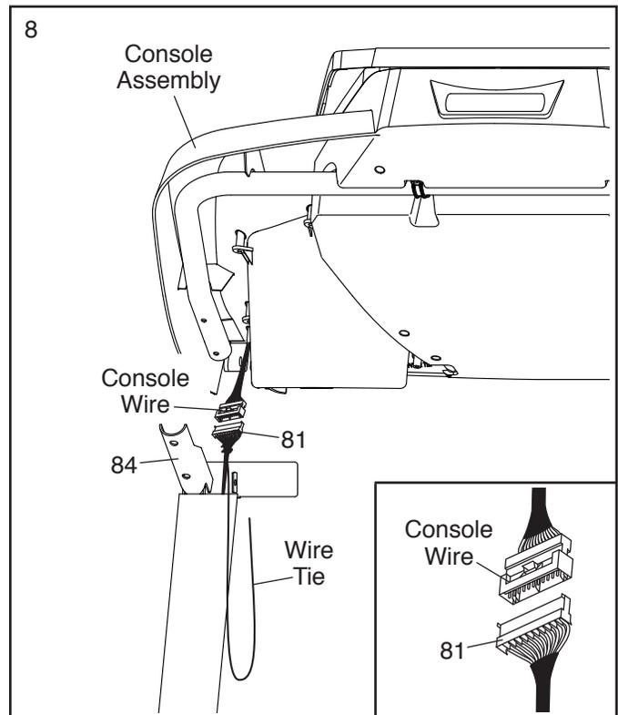
9. Set the console assembly on the Handrails (84). **Be careful not to pinch any wires.** Insert the excess Upright Wire (81) into the Right Upright (90).
