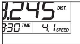
The upper display can show the elapsed time, the distance that you have walked or run, the approximate number of calories you have burned, or the speed of the walking belt. Press the Priority Display button repeatedly until the upper display shows the information that you are most interested in viewing. Note: While information is shown in the upper display, the same information will not be shown in the lower left or lower right display.
