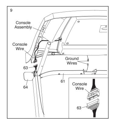
10. Insert the wires into the Right Handrail (64) through the indicated hole as you set the console assembly on the Left and Right Uprights (66, 76). **Make sure that no wires are pinched.**
