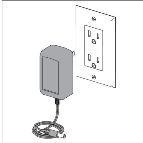
2. Plug the battery charger into a wall power outlet. The light on the charger housing should illuminate. Red LED light indicates battery is charging and a green LED light indicates battery is fully charged.
