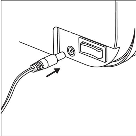
1. Make sure power switch is in the OFF position before plugging in the charger. Insert charger into charging port on the right side of the battery box.
