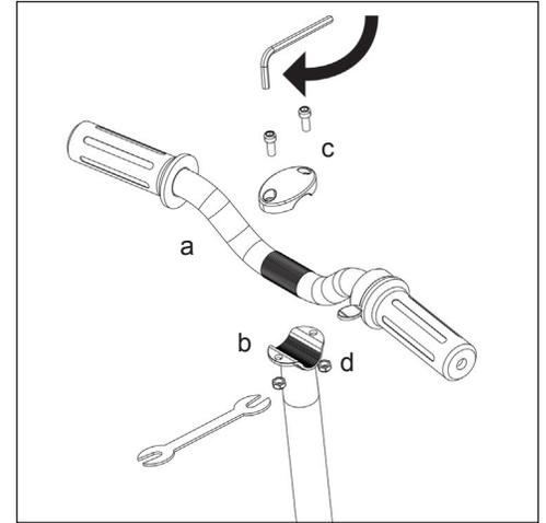
3. Align handlebars both vertically and horizontally (a) onto handlebar steer tube clamp (b) install handlebar clamp and hardware (c&d) and tighten evenly and securely with the 5mm hex wrench and 10mm wrench.
