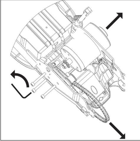
4. If replacing the chain, remove the motor bolts with a 4mm hex wrench. Slide motor out of the frame slightly so that there is enough room to remove/replace the chain onto the motor gear. Replace spacers and retighten bolts.
