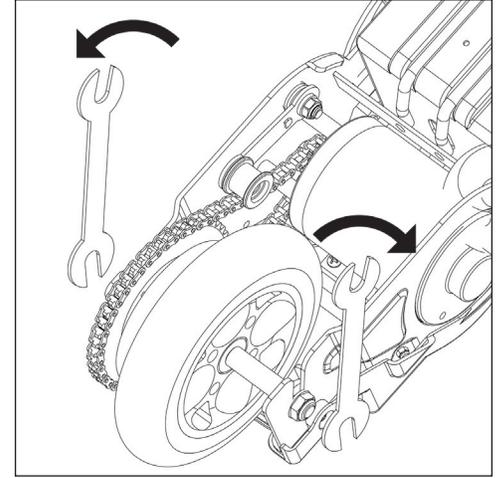
6. Ensure axle washers are seated correctly against the frame. After tightening axle nuts with 13mm wrenches check wheel alignment and the tracking of the chain by rotating the wheel counter clockwise with your hand. Wheel should spin freely and easily.
