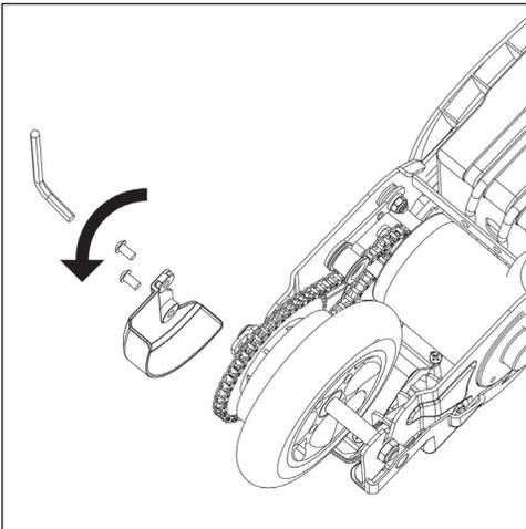
7. Reinstall chain cover with a 4mm hex wrench. Do not over tighten bolts.
