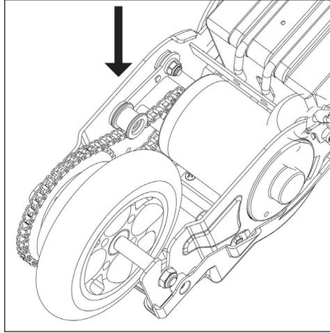
5. Place the chain under tensioner wheel and onto the rear chain wheel gear and install replacement wheel into the frame. Do not tighten axle nuts yet.
