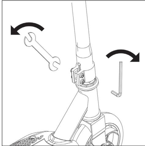
2. Tighten the bolts with the 5mm hex wrench and 10 mm wrench. Tighten bolts evenly and securely.
