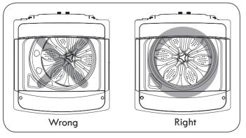
3. To make sure that the washer is properly level, open the lid and look from above to see if the tub is centered. If the tub is NOT centered (as shown in the drawing on the left), readjust the feet. If you have a level, check your washer with the level.
