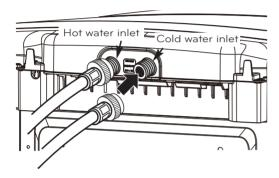
1 Turn OFF both water faucets completely. Unscrew the hot and cold water lines from the back of the washer.
