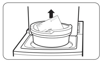
2. Save the foam block for future use. If the washer must be moved in the future, this will help prevent damage to the washer during transportation.
