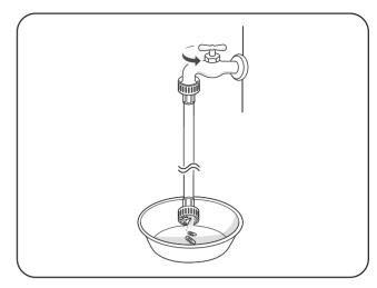
3. Always run a gallon or two of water through each inlet hose to flush dirt, scale and other debris out of the water lines. Doing so will help prevent future problems with clogged filter screens, and will also allow you to verify which hose is hot and which is cold.
