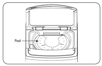
**3.** Carefully remove the two foam pads which cover the top sides of the tub guide, making sure not to leave behind any pieces of the foam.
