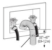
If the water valves and drain are built into the wall, fasten the drain hose to one of the water hoses with the cable tie (ribbed side on inside).
