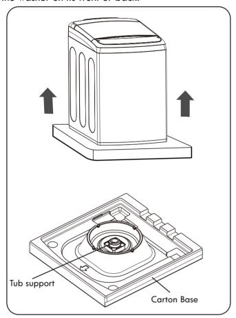
After removing the carton and shipping material, lift the washer off the foam base. Make sure the plastic tub support comes off with the base and is not stuck to the bottom of the washer.
