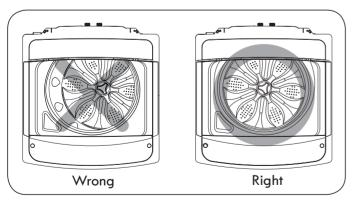
3. To make sure that the washer is properly level, open the lid and look from above to see if the tub is centered. If the tub is NOT centered (as shown in the drawing on the left), readjust the feet. If you have a level, check your washer with the level.
