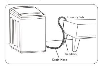
Bend the end of the drain hose to the desired shape and support it on the edge of the laundry tub. Use a tie strap to secure the drain hose in place.
