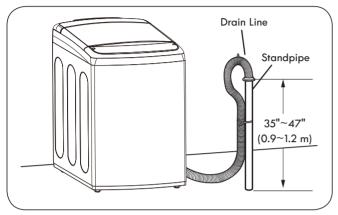
Bend the outlet end of the drain hose to form a U shape. Insert the end of the drain hose into the drain. If the drain is large enough for the flange on the hose to fit inside, then do not insert the flange more than 1-2 inches into the drain. Use the tie strap included with the installation materials in the foam block in the tub to secure the drain hose to the drain.
