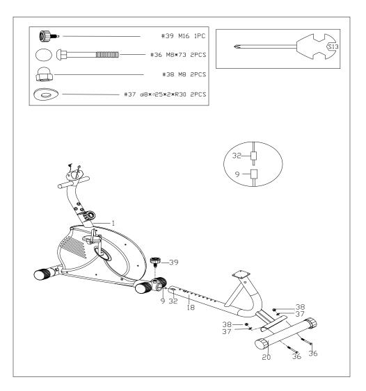
a. Secure Rear stabilizer (20) to Seat rack combine (18) with Bolts (36), Arc washers (37) and Nuts (38);
