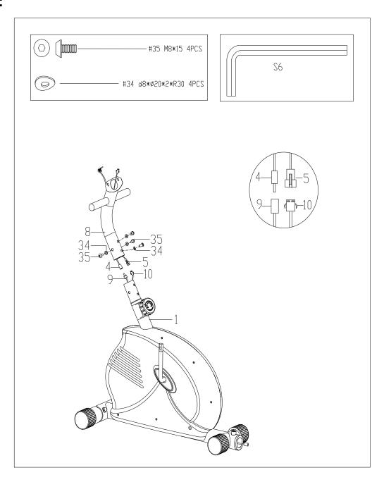
a. Connect Hand pulse wire 1 (4) with Hand pulse wire 2 (9), Trunk wire (5) with Sensor wire (10);
