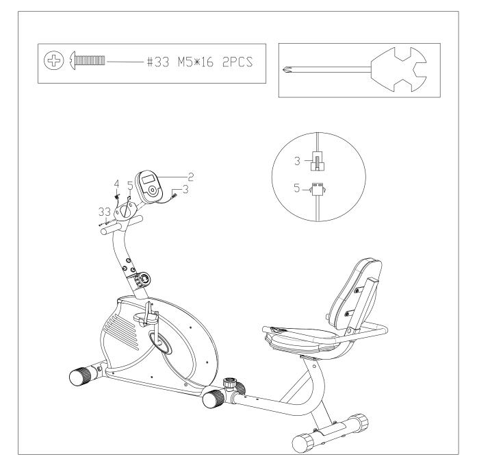
Connect Trunk wire (5) with Computer wire (3), and secure Computer (2) to Handlebar post (8) with Screws (33). Then insert Hand pulse wire 1 (4) to the hole on the back of computer. Assembly is complete.
