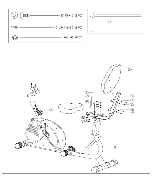
a. Secure Cushion bracket (24) to Seat rack combine (18) with Bolts (35), Spring washers (42) and Washers (40);
