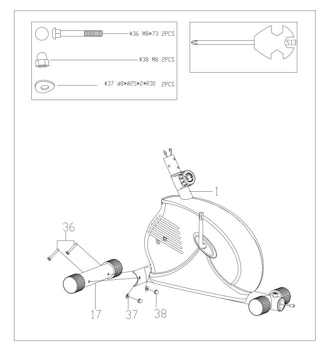
Secure Front stabilizer (17) to Main frame (1) with Bolts (36), Arc washers (37) and Dome nuts (38).
