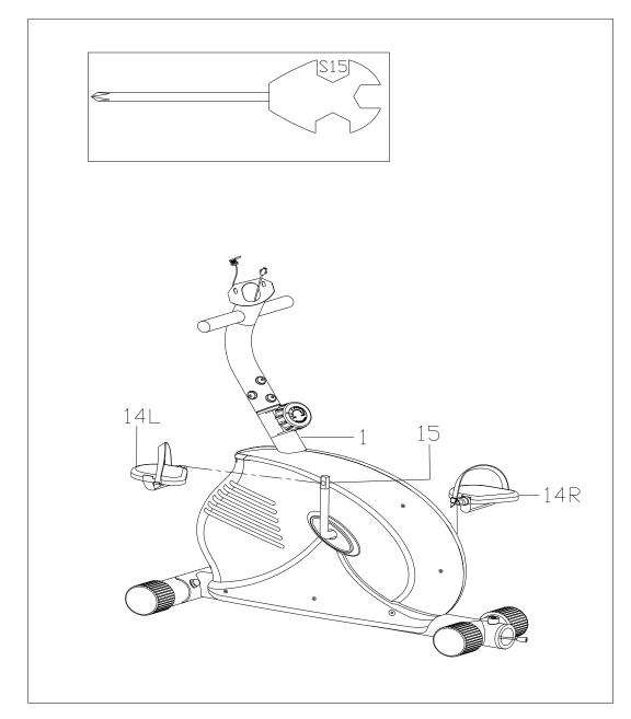
Secure Pedals (14L/R) to the Crank (15) on the Main frame (1).
