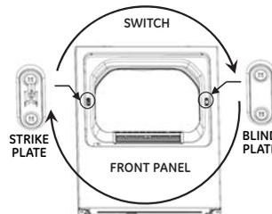
**4** Rotate the door 180°. Insert it on the opposite side of the opening by moving the door **IN** and **DOWN** until the top hinge and the bottom hinge are resting on the top screws inserted in step 1.
