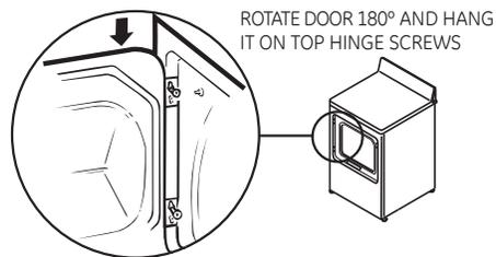
**5** Remove the remaining screws from the side of the opening from which the door was removed. With these screws, secure each hinge at the bottom. Tighten the two top screws of each hinge. Reinsert the plastic plugs on the side from which the door was removed.
