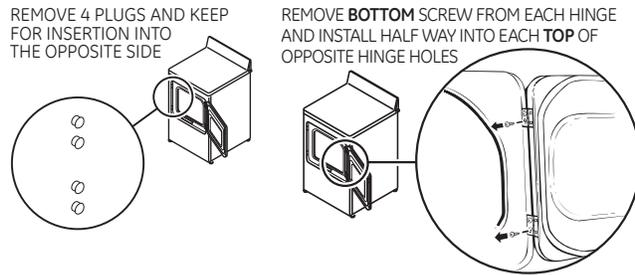
**2** Loosen top screw from each hinge on the dryer face half way. With one hand holding the top of the door and the other hand holding the bottom, remove the door from the dryer by lifting it **UP** and **OUT**.
