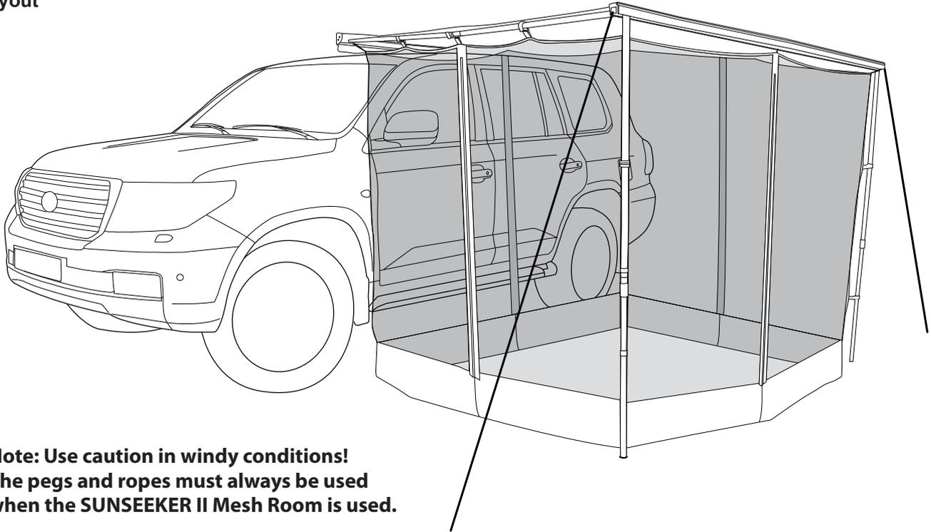
The SUNSEEKER II Mesh Room is to be used in conjunction with SUNSEEKER I or SUNSEEKER II awnings. Holes may need to be drilled on these models. Models with the black sticker as shown (on the right) do not need to have any holes drilled.
