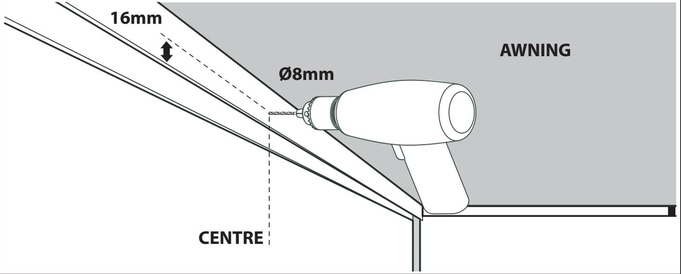
**04** Drill 3 x 8mm holes from the bottom as shown. DO NOT drill all the way through both wall sections.
