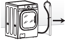
Connecting the drain line
