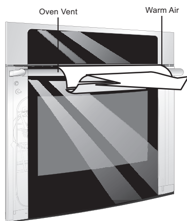
Figure 1: Oven vent location
