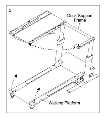
3. Rotate the desk to the right. Then, raise the right side of the desk so that the latch pin will seat fully into the catch. **IMPORTANT: The treadmill will not function if the latch pin is not properly seated.**
