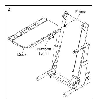
3. Rotate the desk to the right. Then, Raise the right side of the desk so that the latch pin will seat fully into the catch. **IMPORTANT: The treadmill will not function if the latch pin is not properly seated.**
