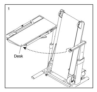
Hold the frame firmly with your right hand while pressing the platform latch to the left with your left hand. Then, lower the platform to the floor.
