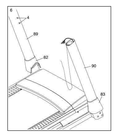
Identify the left handrail assembly (B). Attach the left handrail assembly to the Left Upright (89) with two 5/16" x 2 1/2" Screws (28) and two 5/16" Star Washers (11). Do not fully tighten the Screws yet.
