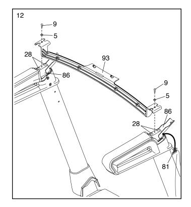
13. With the help of a second person, hold the console assembly near the Handrails (86) (only one side is shown).
