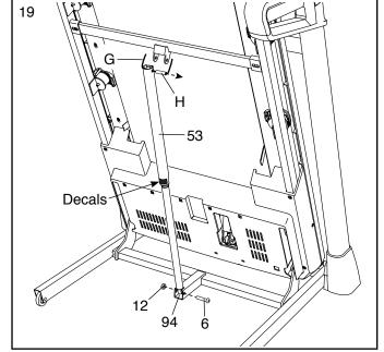
20. Attach the upper end of the Storage Latch (53) to the bracket on the Latch Crossbar (38) with a 5/16" x 2 1/4" Bolt (3) and a 5/16" Nut (12).
