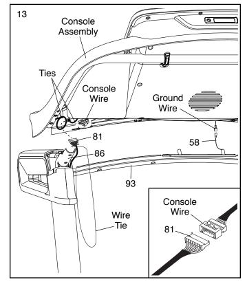
14. Set the console assembly on the brackets on the Handrails (86). **Make sure not to pinch any wires.**
