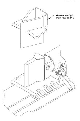
To install 4-way wedge, simply slide it over the top of the log splitter wedge ensuring it is fully seated. Ensure appendages are safe from any pinch points during installation.
