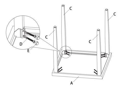
**Step 2:** Check and make adjustment as needed, make sure all the bolts were fully tightened. Place the ceramic table top on the frame gently.
