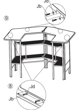
· Note: adjust the "U"shaped connector and aline the holes
