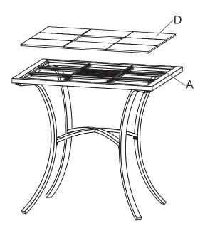
• Securely tighten all bolts in a digonal pattern.
