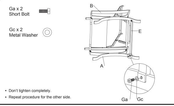
**4** Pushing the front seat into the rear seat and back
