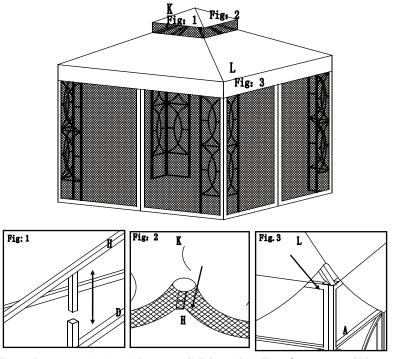
Fig.1: Remove the Arch Beam 1 (H) from Big Top Connector (D), put Big Canopy (L) onto Big Top, but don't spread fully, then put the Arch Beam 1 (H) onto the Top Connector (D).
