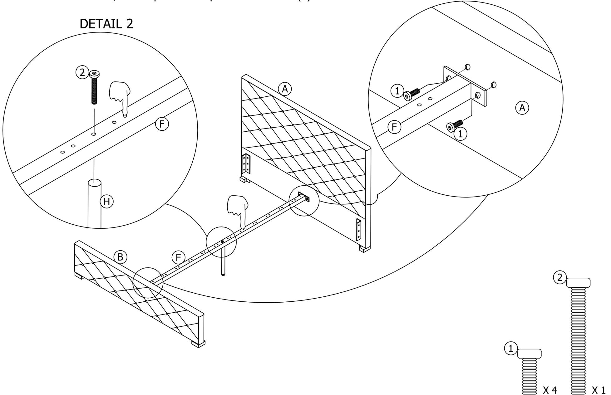
**4** Attach part "C" to part "A" with bolt (1), as shown below.
