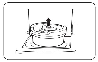
2. Save the foam block for future use. If the washer must be moved in the future, this will help prevent damage to the washer during transportation.
