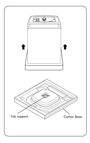
1. After removing the carton and shipping material, lift the washer off the foam base. Make sure the plastic tub support comes off with the base and is not stuck to the bottom of the washer.
