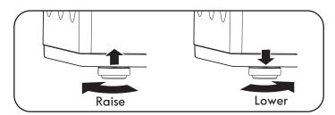
**2.** Adjust the leveling feet. Turn clockwise to raise the washer or counterclockwise to lower it.
