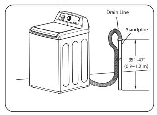
Bend the outlet end of the drain hose to form a U shape. Inset the end of the drain hose into the drain. If the drain is large enough for the flange on the hose to fit inside, then do not insert the flange more than 1-2 inches into the drain. Use the tie strap included with the installation materials in the foam block in the tub to secure the drain hose to the drain.
