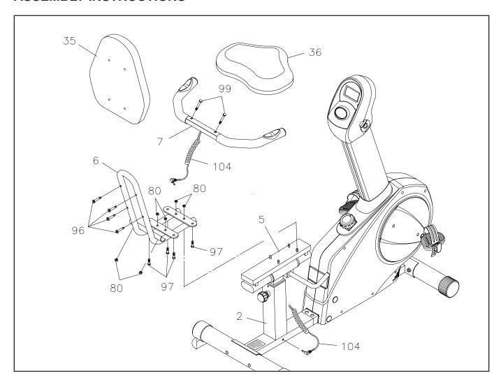
**NOTE:** Be careful not to damage the **PULSE SENSOR WIRES(104)** while doing assembly Step 8 and Step 9.
