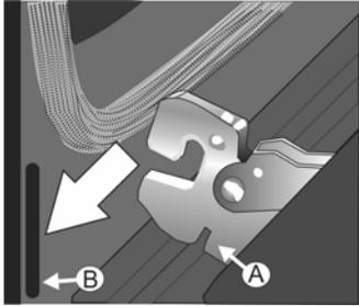
1. Holding the door firmly in both hands, place hinges in hinge slots.
