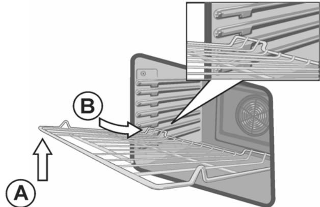
4. Bring the rack to a horizontal position. Push the rack all the way in. The rack should be straight and flat. It should not be crooked.
