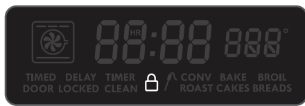
Figure 7: Cooktop lockout indicator
