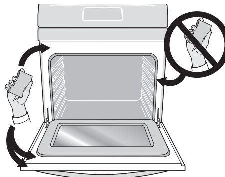
Figure 33: Oven door area to clean and not clean (gasket).
