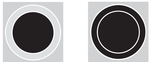
Figure 6: Dual burner set to single (L) and double (R).
