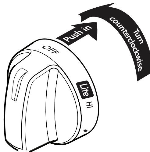
Figure 7: Correct way to set burners
