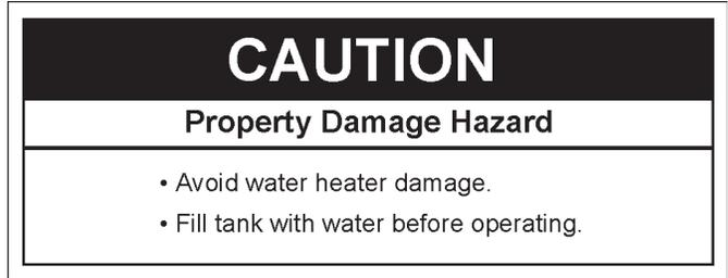
Never use this water heater unless it is completely full of water. To prevent damage to the tank and heating element, the tank must be filled with water. Water must flow from the hot water faucet before turning "ON" power.
