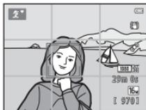
In addition to information shown with **Auto info**, a framing grid is displayed to help frame pictures. The framing grid is not displayed when recording movies.
