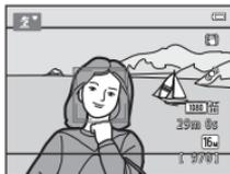
In addition to information shown with **Auto info**, a frame that represents the area that is captured when recording movies is displayed before recording begins. The movie frame is not displayed when recording movies.
