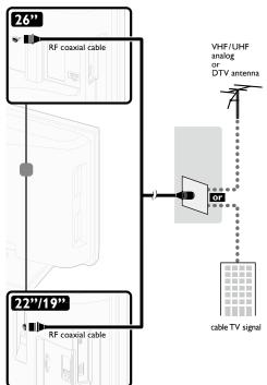
Once connections are completed, turn on the unit and begin initial setup. Channel scanning is necessary for the unit to memorize all available channels in your area. [Initial Setup]
