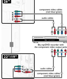
The unit accepts 480i/480p/720p and 1080i of video signals for this connection.
