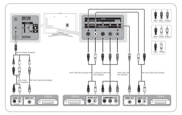
S For better picture quality, we recommend the Component connection over the A/V connection.
