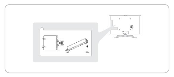
This socket is designed to accept an extension device called the Evolution Kit. The Evolution Kit enables the TV to run a variety of the latest applications for a better user experience.
