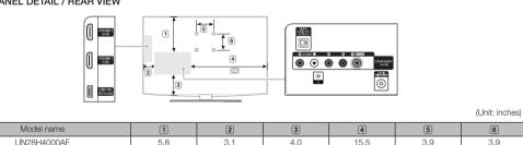
UN28H4000AF 5.8 3.1 3.9 NOTE: All drawings are not necessarily to scale. Some dimensions are subject to change without prior notice. Refer to the dimensions prior to performing installation of your TV. Not responsible for typographical or printed errors. © 2014 Samsung Electronics America, Inc
