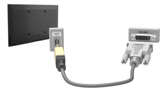
Once the connection has been made, press the **SOURCE** button to select the connected external device.
