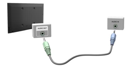
Once the connection has been made, press the **SOURCE** button to select the connected external device.
