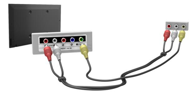
Once the connection has been made, press the **SOURCE** button to select the connected external device,
