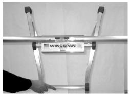
4. Make sure the WingSpan is centered and securly on the top rung.
