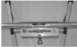
This is how the WingSpan Wall Stand Off should look after you have assembled it and placed it correctly on the top rung when the ladder is in extension form.
