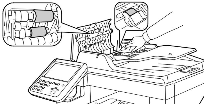
**Note:** If the duplex automatic document feeder feed rollers and separation pad get stained with toner or debris, they can cause stains on the documents. To remove stains, use a soft lint-free cloth dampened with a neutral detergent or water.
