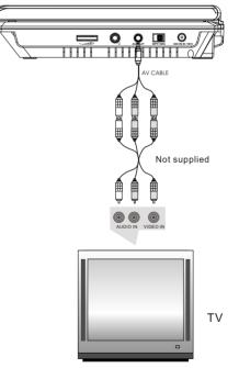
Please use AV cable to connect the machine and the TV. Make sure it is connected correctly.
