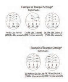
All other torque values must be converted to these units first: \*Foot Pounds can also be obtained by dividing Inch Pounds by 12
