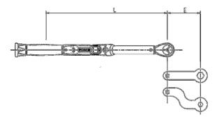
E – Effective Length of extension measured along the center line of the torque wrench
