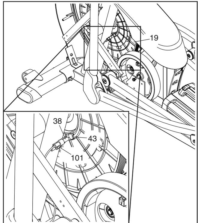
Next, loosen, but do not remove, the indicated M4 x 16mm Screw (101). Slide the Reed Switch (38) slightly closer to or away from the Magnet (43), and then retighten the Screw.
