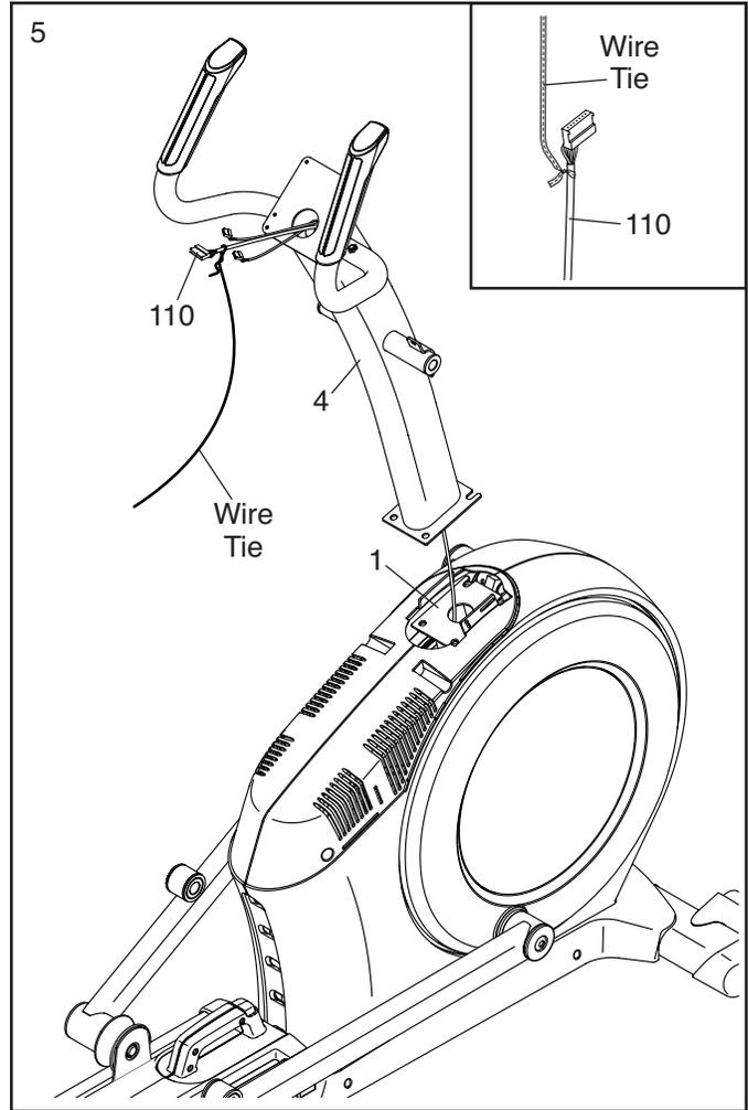
6. **Tip: Avoid pinching the Upper Wire (110). Avoid damaging the indicated plastic tabs.** Have a second person hold the Upright (4) on the Frame (1).
